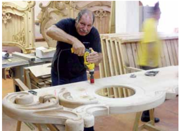
Allen Velthoen cutting light socket holes in John's façade.
