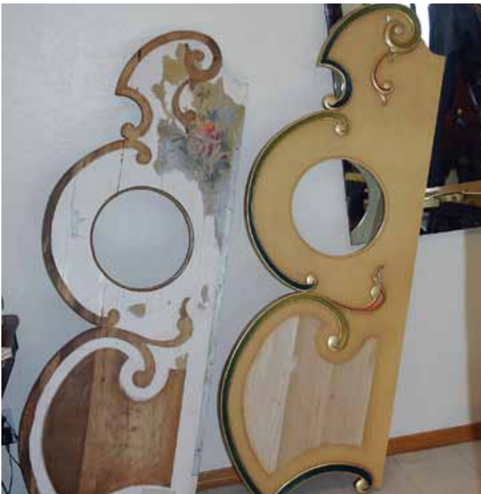
Left wing panels, original, and new, with transferred carvings. The new wings are made exactly as the factory did with a poplar substrate core with 1/8" cross banding. No plywood or other modern materials are used anywhere in the project.
