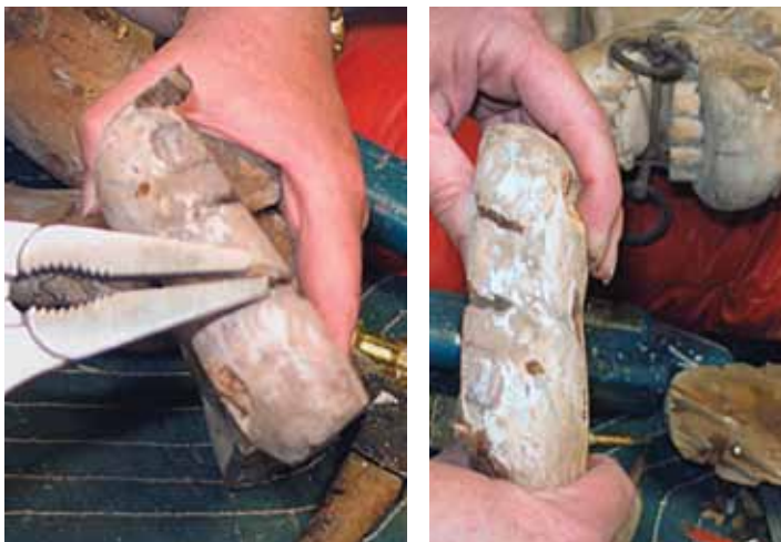
PHOTO B7 - Use vice grips or a nail puller to work the rest of the fastener out of the joint (left). PHOTO B8 - The fasteners are gone (right).
