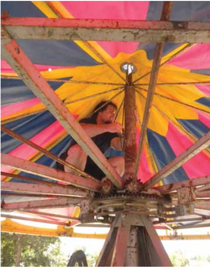
Our oldest grandson raising the canopy. This photo also gives a good look at the upper gear, the gears and crank rods, the various metal braces and sweeps, and the brushes for the electrical pickup for lighting.
