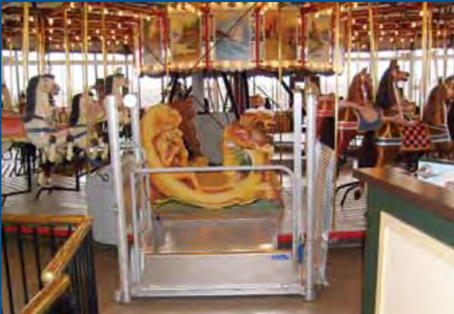
Adaptive Engineering's portable wheelchair lift at the New York State Museum in Albany, NY. The lift services the 1915 Herschell-Spillman carousel.
