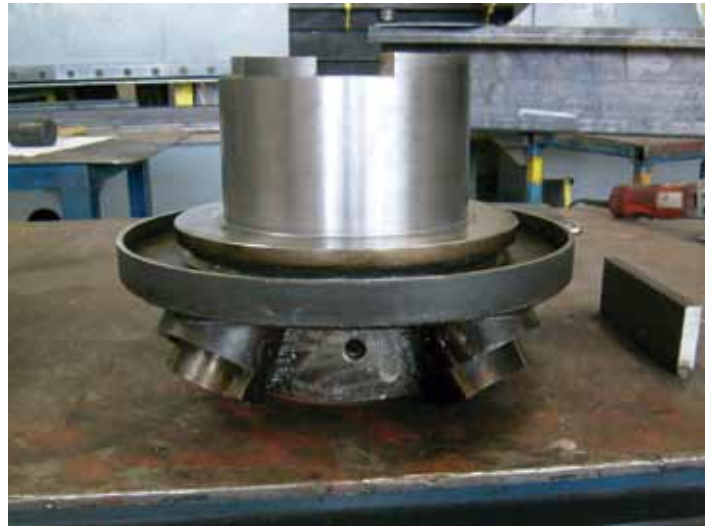
Shown above and right, center hub bearing for the Fond-Du-Lac carousel. The original brittle cast iron one (shown left), the new steel replacement behind it and close up (right).
