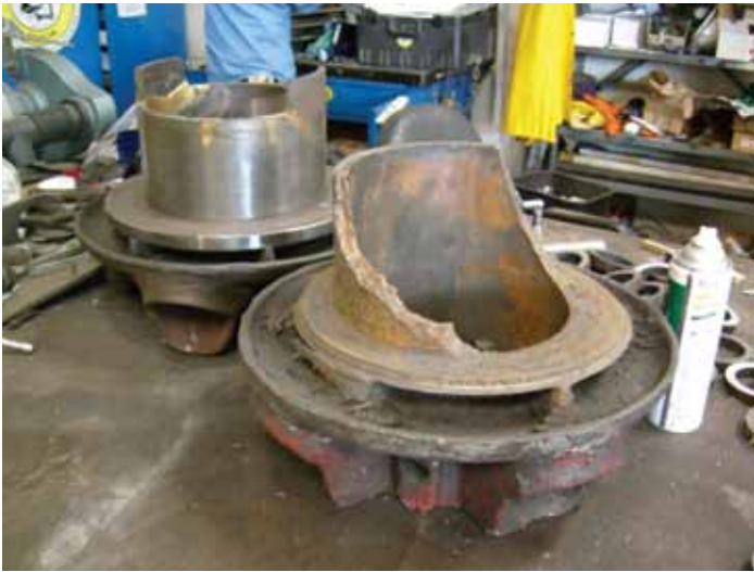
Shown above and right, center hub bearing for the Fond-Du-Lac carousel. The original brittle cast iron one (shown left), the new steel replacement behind it and close up (right).
