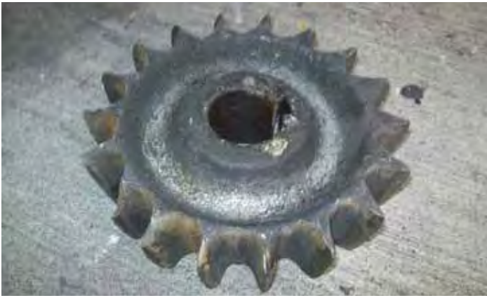
Original worn out pinion gear.
