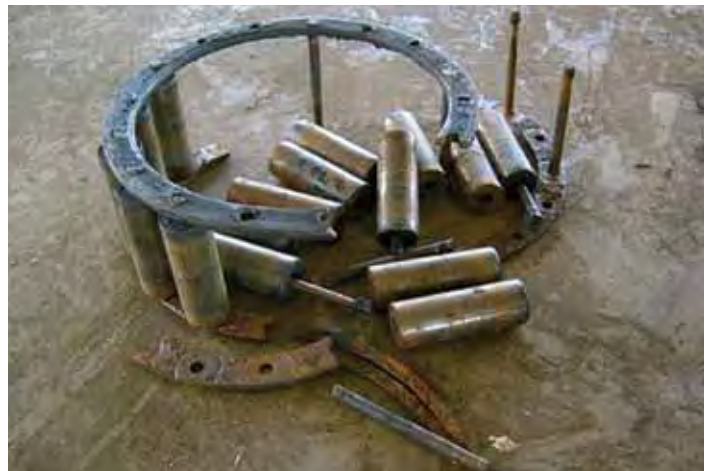
The original center bearing from the Roswell 1927 Spillman carousel shows 80 years of wear.
