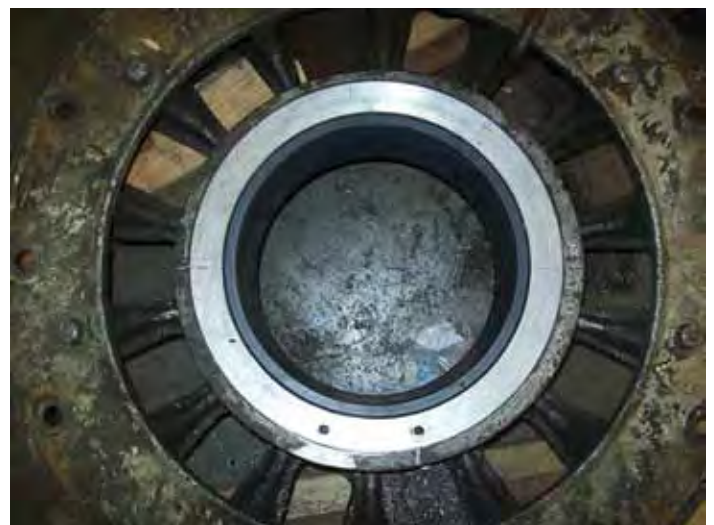
Sweep hub with new steel bushing and Nylatron bearing.
