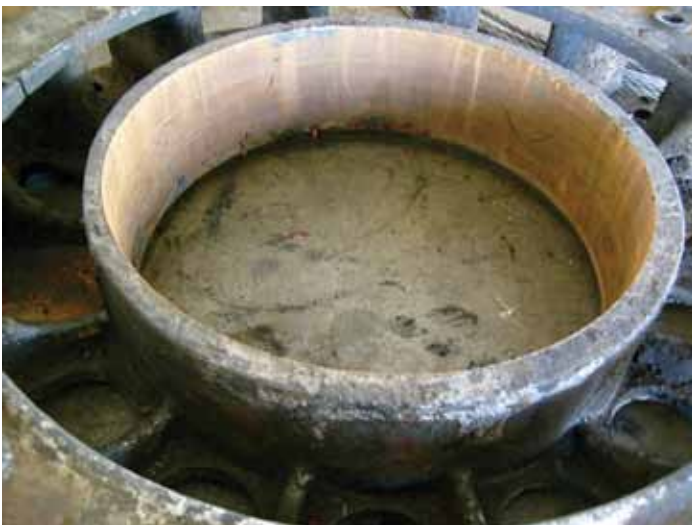
1927 Spillman Engineering sweep hub before repair.
