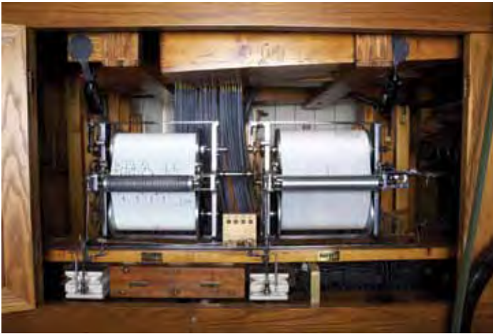
One of the roll frames was modified during restoration in the 1980s to accommodate Wurlitzer 165 rolls as well as the 66-key music rolls.
