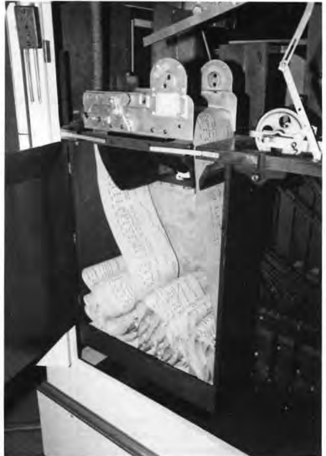
Here is a very rare look at the workings of a continuous (or endless) roll band organ. This North Tonawanda model 191 plays on the Balboa Park Herschell-Spillman menagerie machine.
