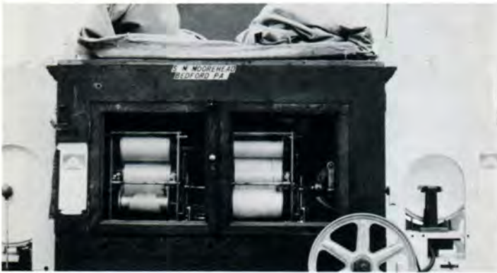
Wurlitzer duplex action with double tracker on a Model 153.
